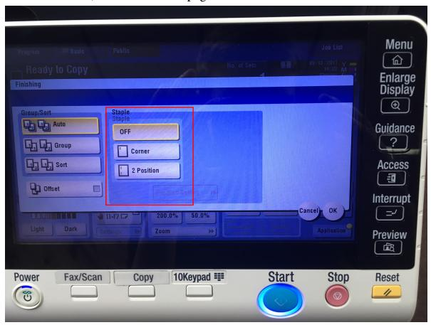
Pictured below is the "Position Setting" menu. Here you can make changes to the way the staples will be positioned. Using the "Original Direction" menu will give you more options and A graphical display of staple position allowing you to make the neccessary changes to get the results you want.
